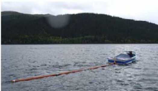
The RTA within a plastic waterproof pipe.
