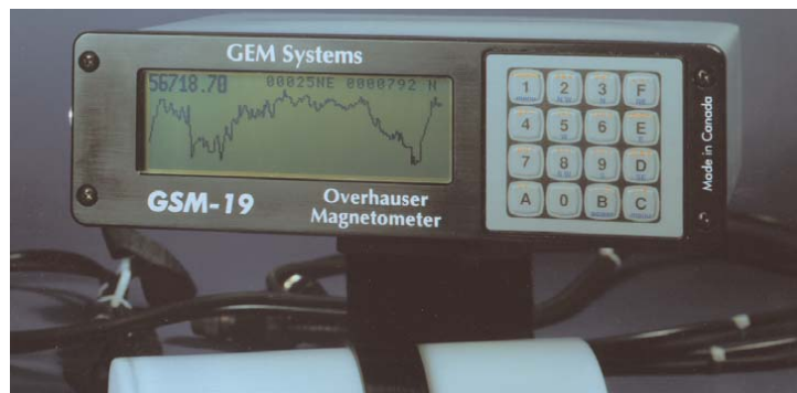
Overhauser (GSM-19) console with sensor and cable. 4 Sensor unit obtains 4 gradiometer (simultaneous) readings in one of two configurations.
