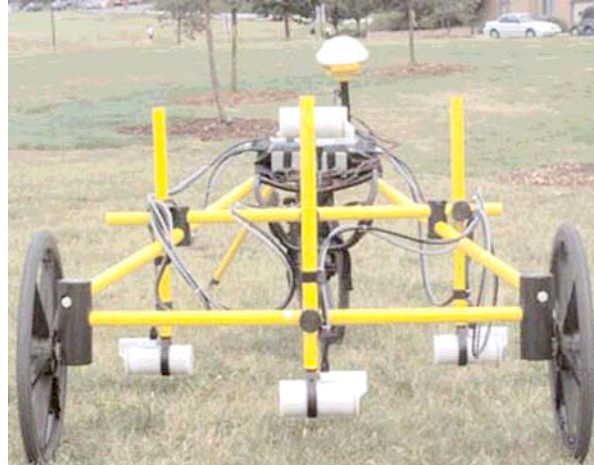
This image of a cart-borne system shows the 3D array in operation. Note that an external GPS is also provided as an option for highly accurate positioning of the survey results
