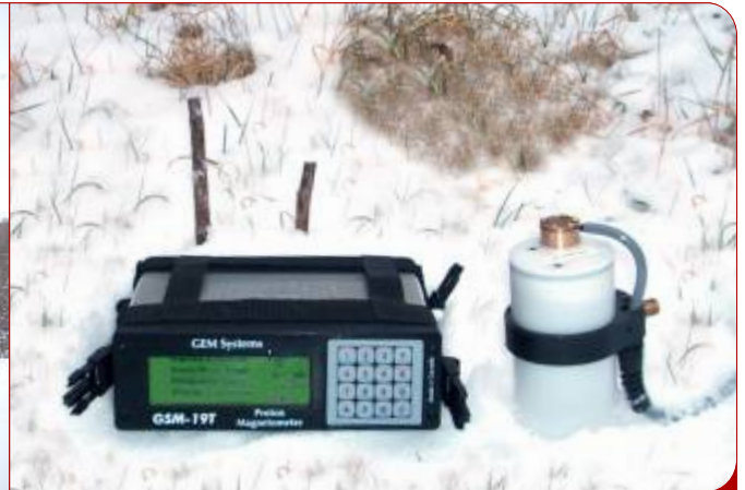
GSM-19T Proton Precession console configured with backpack, additional sensor for gradiometer (simultaneous) readings, built-in GPS and VLF EM system
