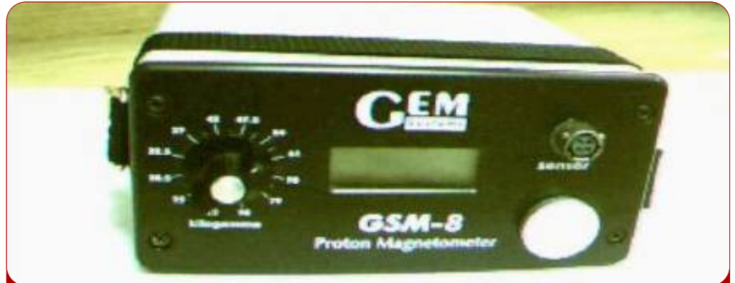
GSM-8 Proton Precession console.
